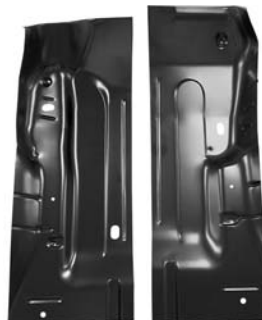
46 1/2"W x 17 1/2"H CAB FLOOR EXT CAB INNR.....1582-221, 222
